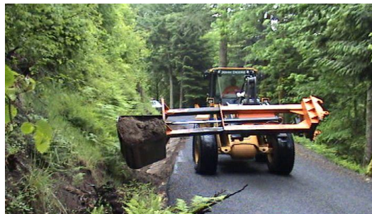
When the bucket is filled with debris (operator can see the bucket filling from the cab by watching viewing hole in the top of the bucket). The Ditchpro can then be lifted and dumped
